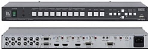
The VP-728 is a 9-input scaler/switcher for analog and digital video, unbalanced stereo, and S/PDIF audio signals. It scales any video signal composite, s-Video (Y/C), component video (YUV), HDMI, computer graphics video and JPEG files) up or down to a selectable graphics or HDTV output resolution via HDMI or 15-pin HD outputs. It provides glitch-free switching between sources through FTB™ (fade-thru-black) switching technology.
